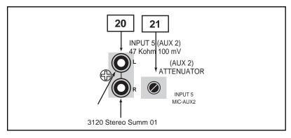
Fig. 15A - Stereo Summing and AUX 2 Input Attenuator
